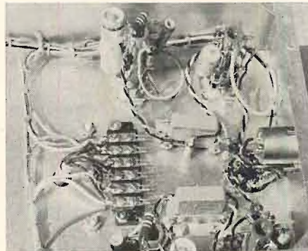
Fig. 7. Arrangement of Vector sockets for amplifier stages.
