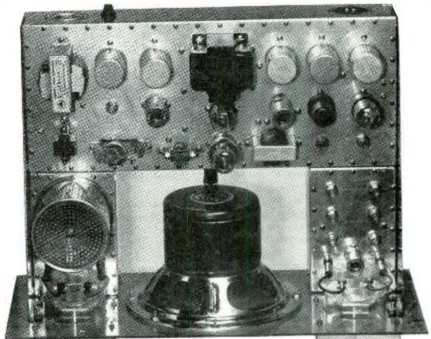
Fig. 3. Rear upper view of monitor, showing three-chassis format used to clear speaker magnet. Wattmeter subchassis is at right, frequency-meter at left, and main chassis at bottom in this view.
