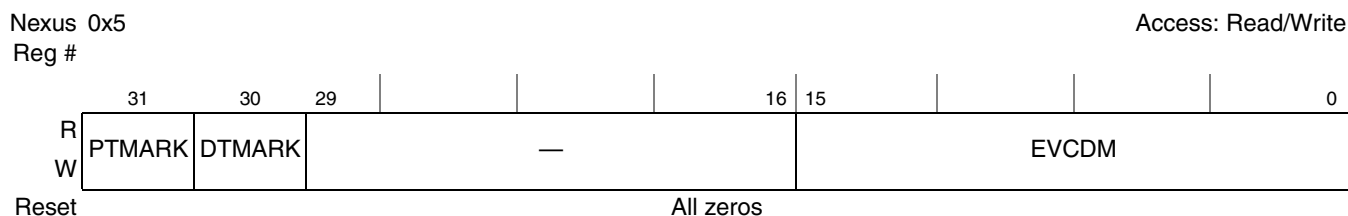
Figure 14-7. Development Control Register 4
