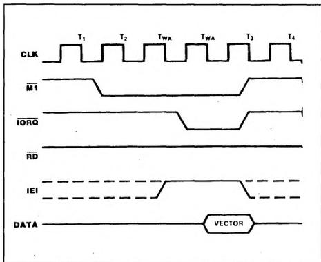
daisy chain enable lines for proper control of nested priority interrupt handling. The CTC decodes the 2-byte RETI code internally and determines whether it is intended for a channel being serviced. Figure 15 shows RETI timing.
