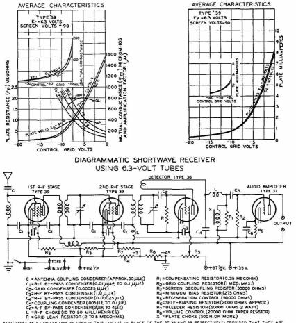
NOTE: TYPES 56, 57 AND 58 MAY BE USED IN THIS CIRCUIT IN PLACE OF THE 37.36 AND 39 RESPECTIVELY, PROVIDED THAT THEY ARE OPERATED AT THEIR RECOMMENDED HEATER, SCREEN, PLATE AND GRID BIAS VOLTAGES. THE SUPPRESSOR GRID OF THE 57 AND 58 SHOULD BE TIED TO THE CATHODE AT THE SOCRET.
