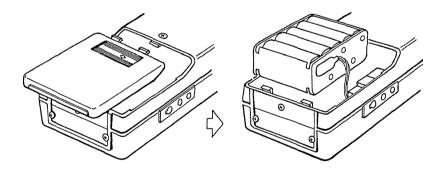
Then switch the transceiver ON by rotating the volume control clockwise and check that the meter needle moves into the red field. If the meter needle does not move, switch OFF immediately and check if the standby-operate-call switch is in the OPERATE position. If this is the case, open the battery compartment to remove the battery holder to ensure that the batteries are correctly in-serted.
